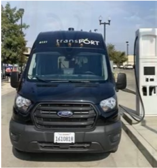
Figure 33: A BE passenger van plugged into a charger
