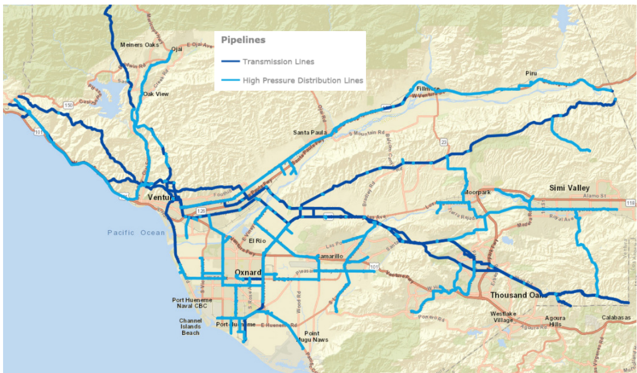
Figure 11: Pipelines in Ventura County
