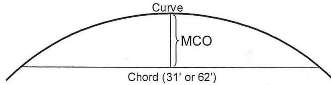
Figure 4. Curve Track Alignment.
