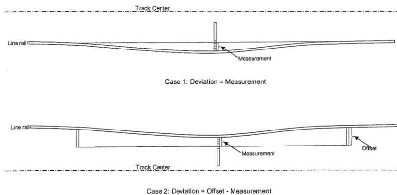
Figure 3. Tangent Track Alignment.
