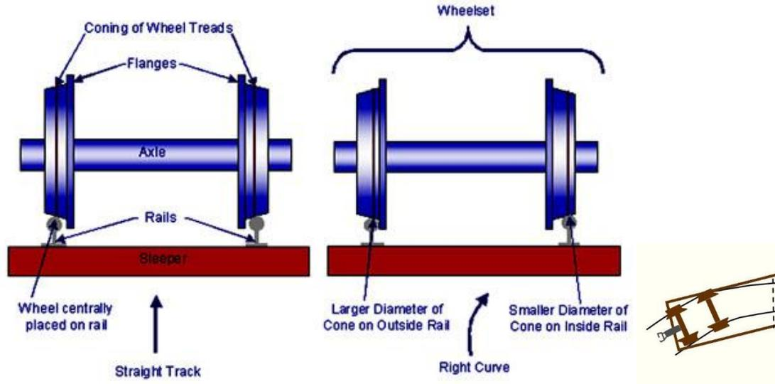
Figure 7. Wheel/Axle assembly.
