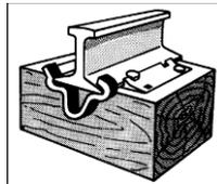
Figure 14 – Rail anchors.
