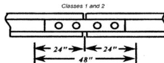
Figure 8. Effective tie under a joint bar.
