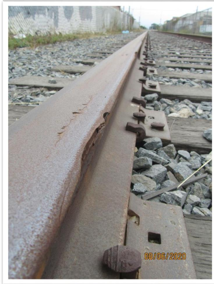
*Image 12. 132# Rail Gauge Side Shell Showing Parent Metal Decay, MP 407.55*
