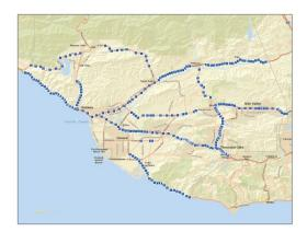
The highway detection system, an Advanced Traveler Information System (ATIS), SpeedInfo, provides incident and speed information to Caltrans District 7's Traffic Management Center (TMC). This information is then fed back to motorists through Caltrans' Changeable Message Signs (CMS) informing motorists of delays and travel times. The cost to operate and maintain the highway detection system is approximately \$153,000 per year.
