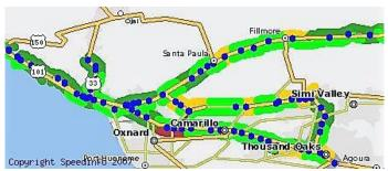
(TMC). The data is then used to detect incidents and predict travel time on segments of the County's road network. The travel time is then used to inform motorists through changeable message signs and L.A. Metro 511. At the present time the sensors are spaced approximately one (1) mile apart and only collect aggregate lane speed.
